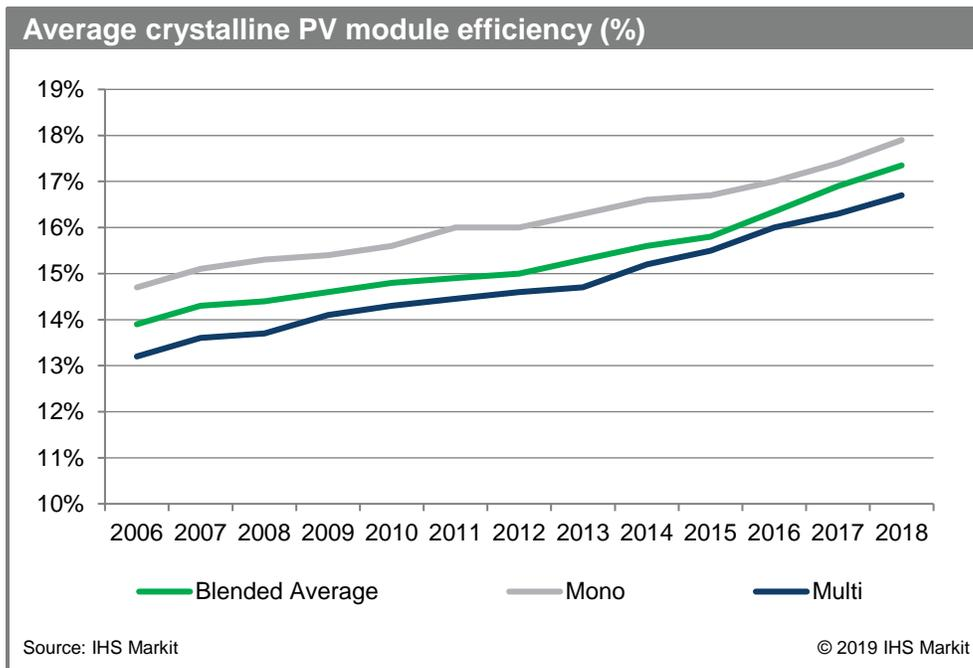
The trend of using monocrystalline cell technology is an increasingly important factor, when it comes to increasing average efficiency. In particular, PERC cells are becoming a mainstream technology, accounting for half of global cell production in 2019, compared to just 14 percent in 2016.
